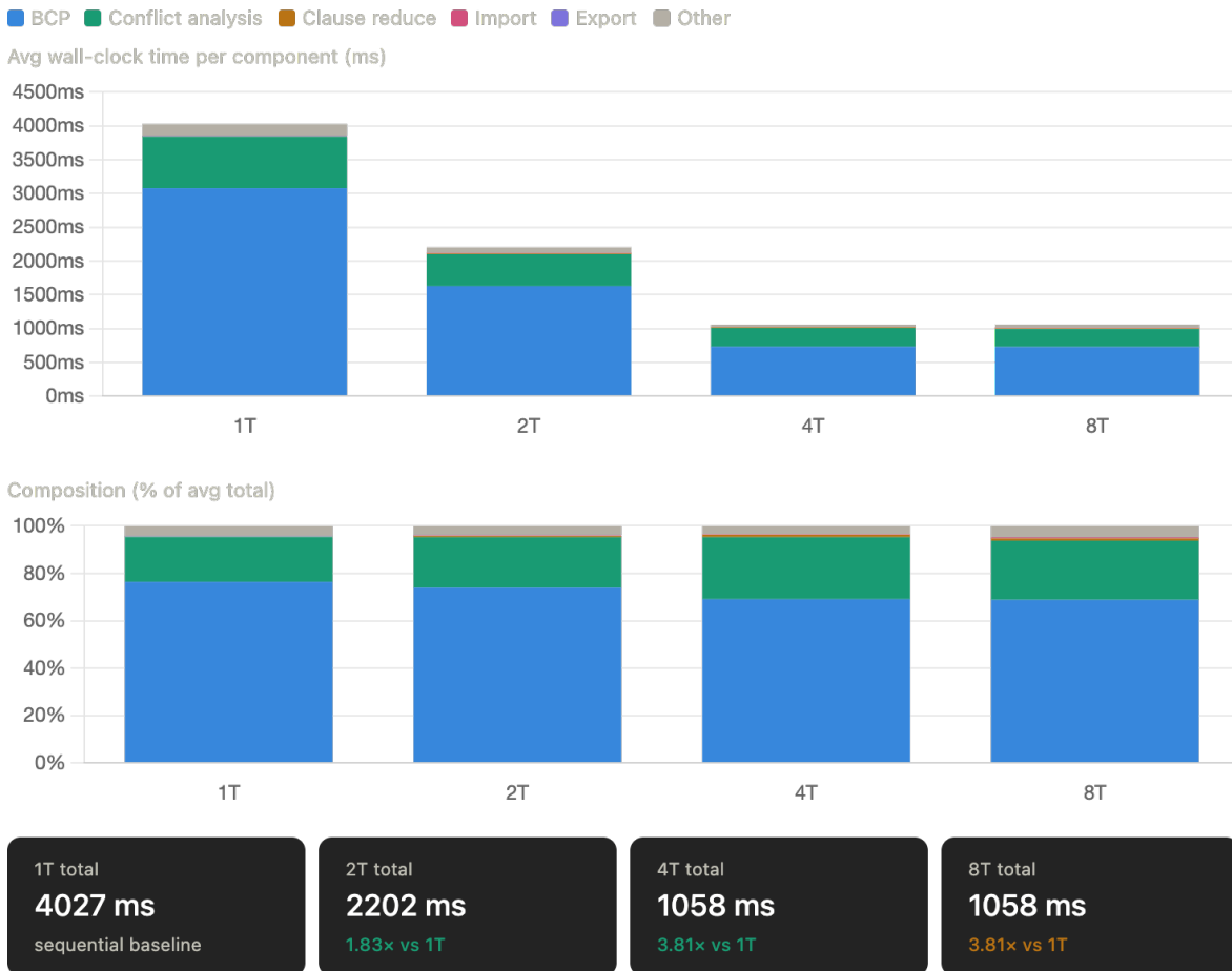
Figure 1: Breakdown of solver time per component, measured via instrumented timing for a representative industrial instance ( tests/uuf150-0100.cnf ).
